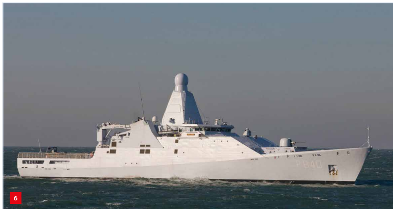
Holland-class ocean-going patrol vessel (OPV) with radars integrated in the superstructure.
