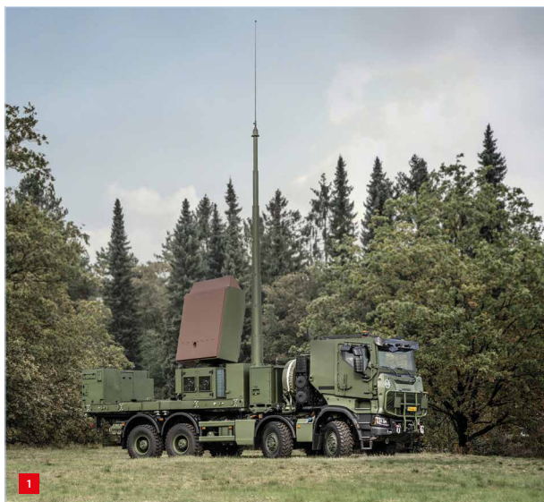
GM200-MM/C mobile multi-mission radar.
