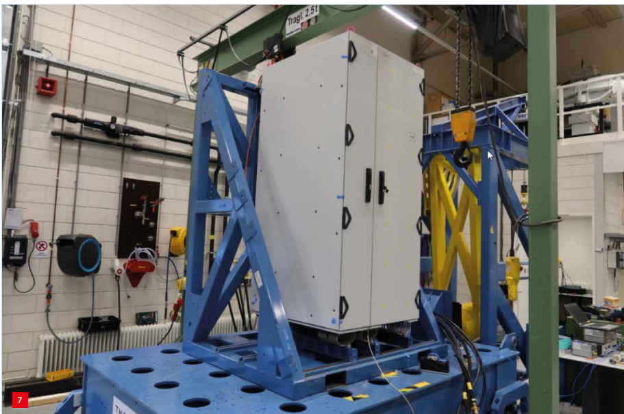
Equipment shock testing at Thales Netherlands.
