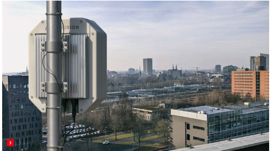
Test of an Aircision system on top of a high building to ensure line-of-sight communication.
