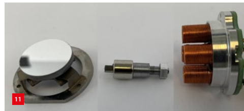
Physical realisation of the beam-steering mirror and the test rig (on the right).
