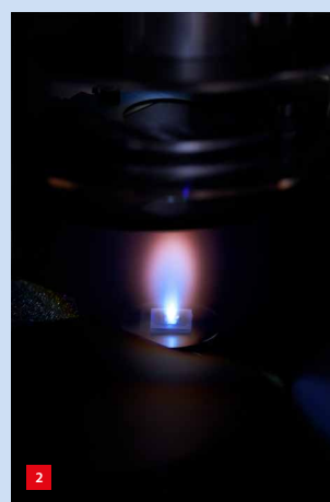
Plasma plume inside the small-area PLD chamber. (Photo: DIFFER / Bart van Overbeeke)
