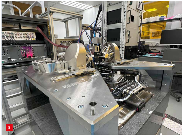
The photonic test prober demonstrator with control cabinets in the background.
