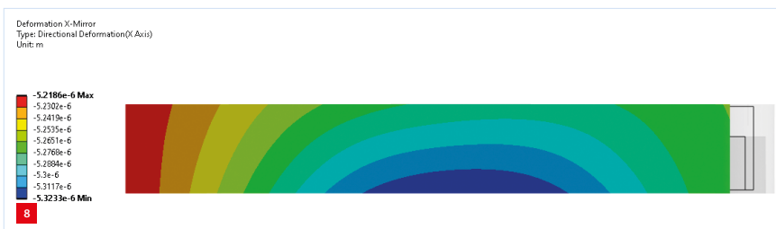
Deformation profile of one of the mirror planes, displaying the x-component of the deformation, which is oriented normal to the plane itself. Scale: -5.3233 \cdot 10^{-6} m (blue) to -5.2186 \cdot 10^{-6} m (red).
