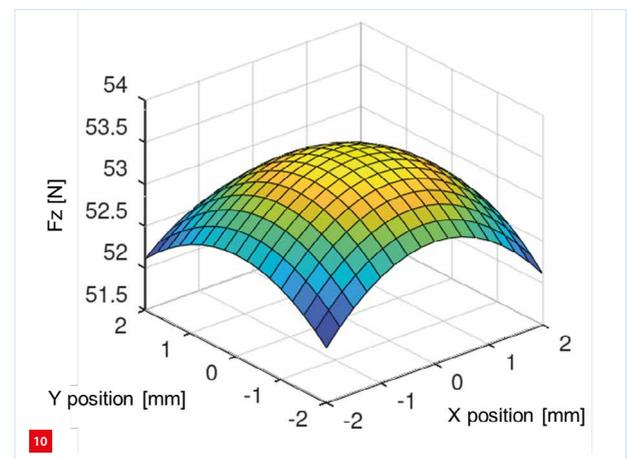
Measured z-force of the gravity compensator over the x,y-stroke.
