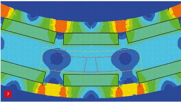
Simulated magnetic field in the actuator.
