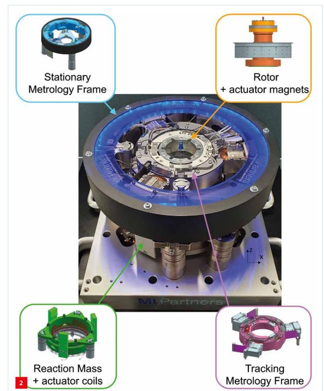
Main system components of the realised MagLev sample manipulator.
