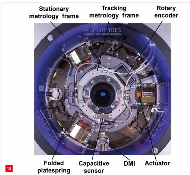
Detailed overview of the in-plane stacked measurement.
