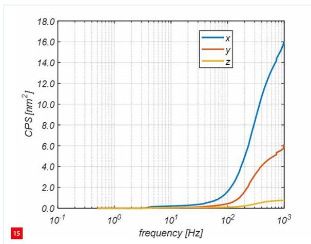
Cumulative power spectrum (CPS) of the servo error.
