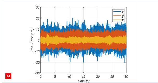
Standstill performance:  $x, y, z$  servo error.
