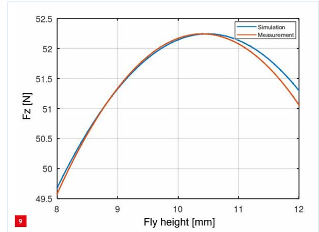
Measured z-force of the gravity compensator over the z-stroke.
