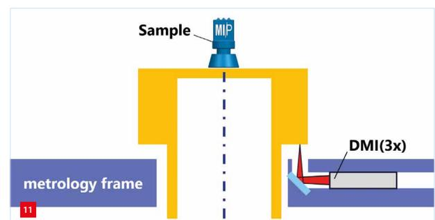
Out-of-plane measurement DMI with 45° mirrors.
