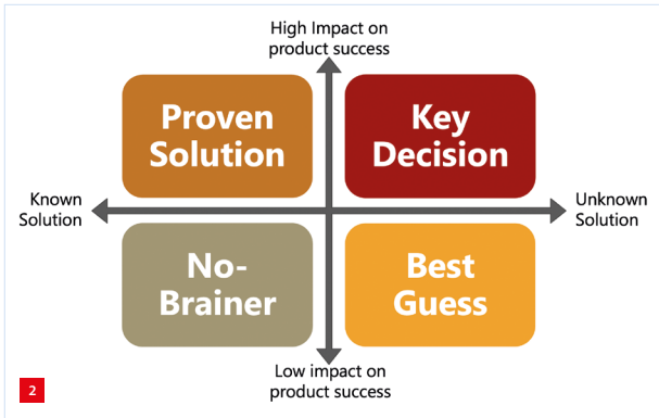
2 Identification of Key Decisions using an assessment based on knowledge of the solution and impact on product success.
