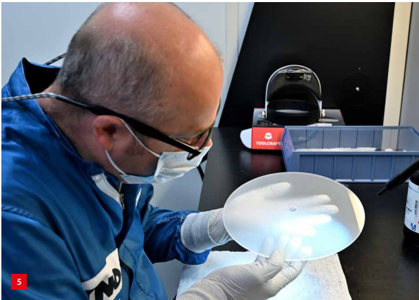
Visual inspection of the mirror shell prior to MRF finishing.
