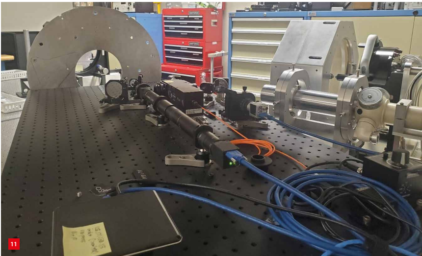
The adaptive mirror on the optical test bench in Hawai'i; in front, the black breadboard contains the wavefront sensors. The small tube is an alignment telescope. The light goes through the circular metal plate on a flat mirror to the Hindle-sphere lens in the hexagonal mount (top right). Next to this, the ASM can be seen with its black housing and the white triangular alignment marker.
