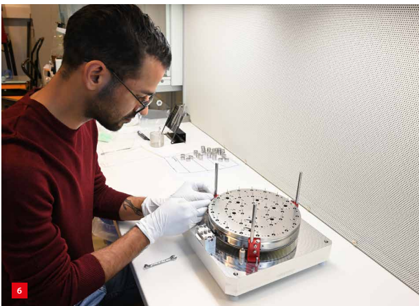
Preparing for the integration of the actuators on the support structure in the integration jig. The thin struts, which are bonded to the mirror shell, can be seen protruding from the top.
