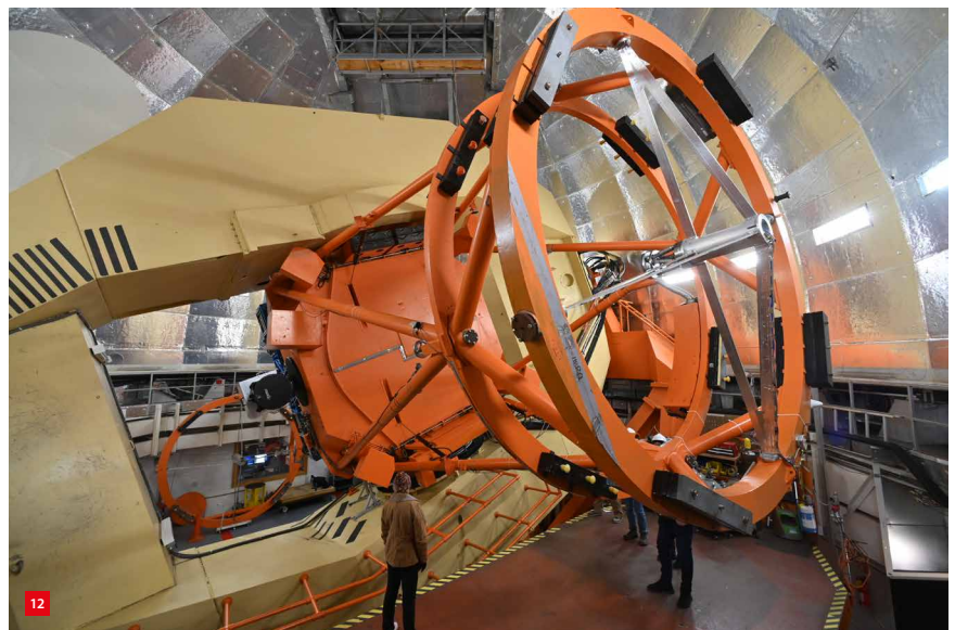
The NASA Infrared Telescope in its dome. The 3-meter primary mirror is just left of the centre, covered with the orange protective covers for the day. A truss structure connects to the large orange ring, the 'top end'. Mounted in the centre of that ring is a long grey tube. The current passive M2, which will be replaced by the ASM, is just visible on the left side of it.
