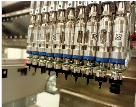
Part of the placement machine, with a close-up of the 10-pipette placement head.
