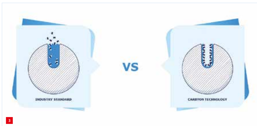
Schematic of the adsorption process: the '3D sorbent' of competitors (left) versus Carbyon's '2D sorbent'.
