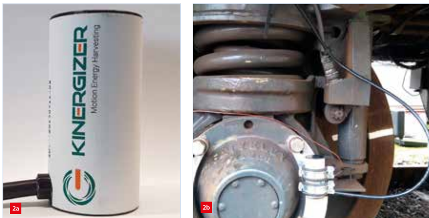
Application example of KinerGizer's energy-harvesting solution. (a) The Hiper-D energy harvester (ø35 mm, 75 mm height, 90 g mass, 1-5 mW power). (b) Mounted to a train bogie axle box.
