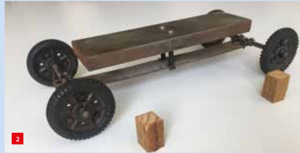
The cart for investigating the influence of the spring suspension. A few wooden blocks could be slid between its parts, to convert the vehicle from suspended to unsuspended.
