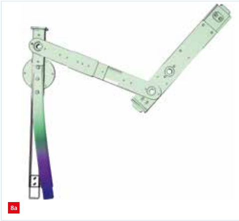
First three in-plane mode shapes from FEA at \theta_1 = 88.2^\circ . The largest displacements of a specific mode shape are shown in dark blue. The representation of the displacements is strongly amplified.
