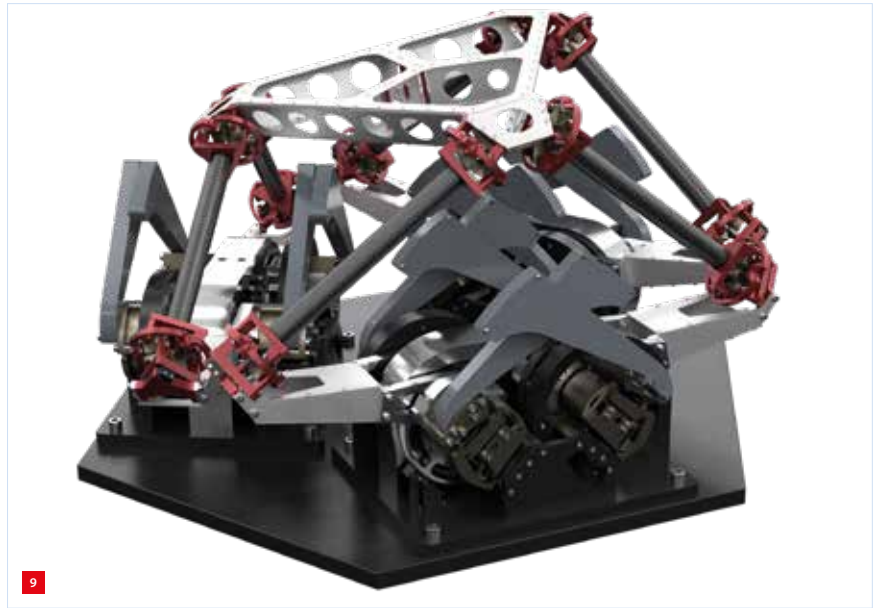
Rendering of the T-Flex in a deflected position, demonstrating the large range of motion.
