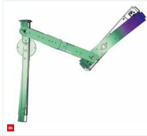
First three in-plane mode shapes from FEA at \theta_1 = 88.2^\circ . The largest displacements of a specific mode shape are shown in dark blue. The representation of the displacements is strongly amplified.
