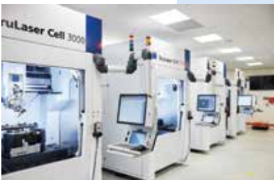
Millux has specialised in the full spectrum of pulsed-laser technologies, including laser welding and laser cutting with Trumpf's TruLaser Cell 3000.
