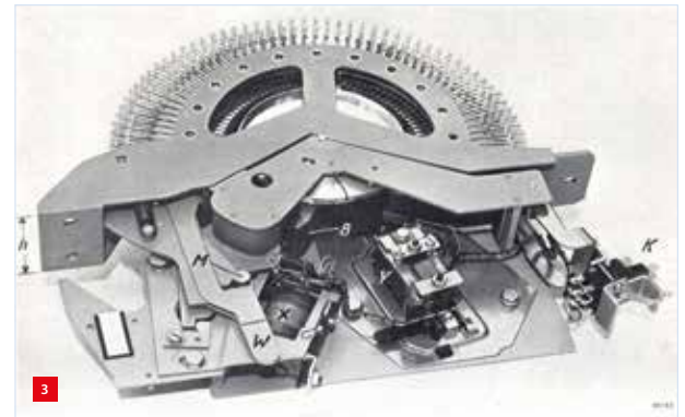
A fast rotary selector for telephony from Philips Telecommunications Industry. The coils for the coupling magnet X (which couples the axis of the contact brushes to a permanently rotating shaft) and the stop magnet Y (which stops the brushes at the desired location) are wound orthocyclically. This application reduced the required electrical power and heat generation in telephone exchanges.
