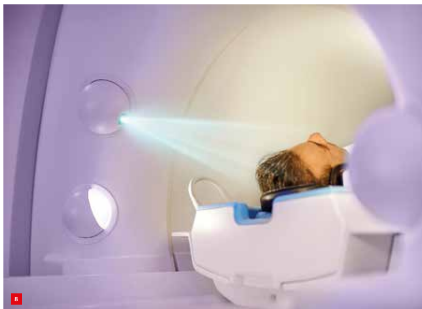
The Philips VitalEye comprises a camera that uses vision software to observe the respiratory behaviour of a patient. Easy hardware? No, this should work in extreme environments, where large magnetic and RF fields could harm the hardware, while the hardware could disturb the quality of the picture or, when coming loose, even harm the patient. Hence, perfect performance on all competencies is needed in development.
