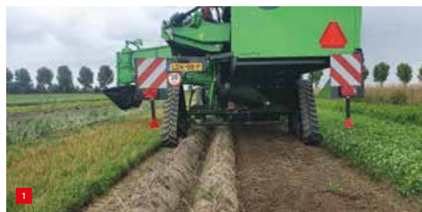
Strip intercropping is combined with controlled traffic farming (CTF) to increase biodiversity and natural predators and to reduce soil compaction. This potato harvester is adapted to the CTF system.
