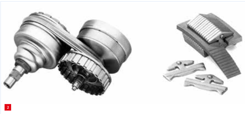
The CVT (left) and a pushbelt, made up of loops and steel elements. (Images courtesy of Bosch Transmission Technology)
