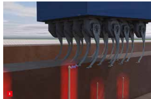
Detection trigger at close proximity of an asparagus spear to a probe.
