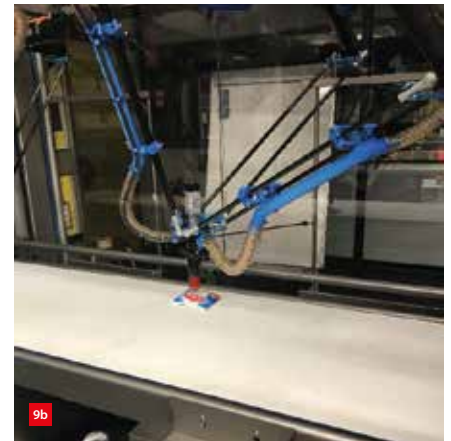
A BPA spider twin delta robot installed at TU/e for research and demonstration purposes in the food-packaging use case.
