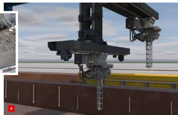
Cutting and extracting asparagus spears from the top of the sand bed. The inset shows a live close-up.
