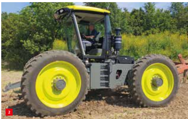
EOX 175, the hydrogen-/electrically powered tractor developed by H2Trac.
