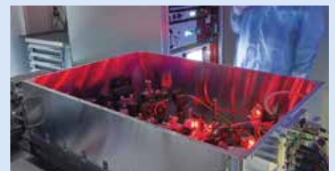
Laboratory prototype for a low-noise quantum frequency converter. (Photo credit: Fraunhofer ILT)
