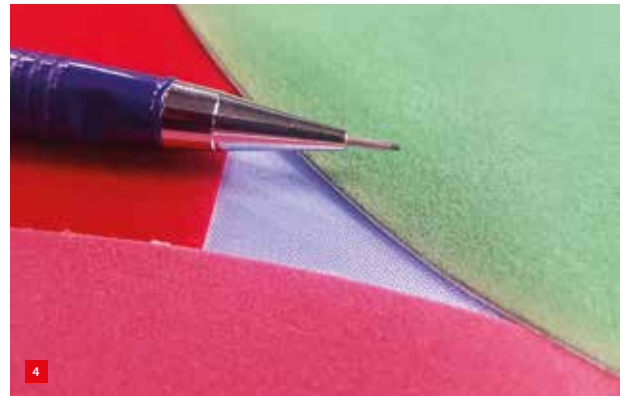
Polishing pads come in a large variety: wool, polyurethane, artificial silk and many more. The hardness and thickness of the pad are important parameters. Different types have their own colour for easy recognition.
