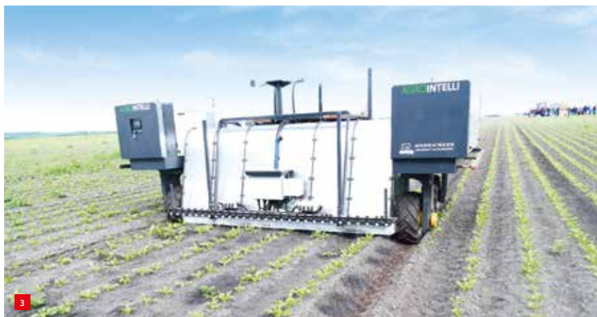
The spot sprayer implement is carried by an autonomous platform.
