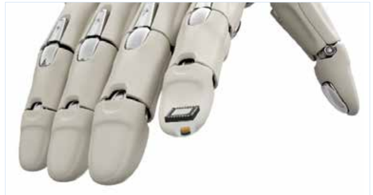
One finger of this robot hand is fitted with the Tactaxis tactile sensor.
