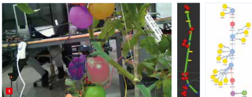
Observations of tomatoes, leaf nodes and fruit nodes (left) are translated into a world model (middle), including a graph-based representation (right).
