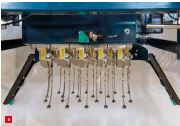
Front view of the detection module. This is a prototype version, featuring four rows of five or six probes each. In the final version, the spacing between the detectors in the lateral direction has been increased, to prevent 'concerted' shoving of the soil by adjacent detectors. This resulted in seven rows of three or four probes each.
