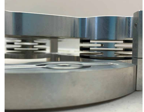
Product wire-eroded with the aid of a fourth axis.
