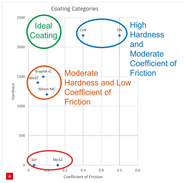
Hardness versus friction coefficient for several counterface (shaft or disc runner) materials in contact with Teflon-coated top foils.
