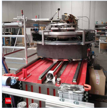
Support structure and rotary table with axial and radial air bearings for an X-ray imaging machine. (a) Overview. (b) Close-up.
