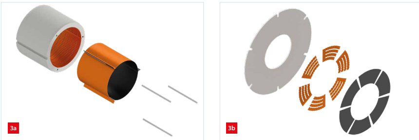
Gas-foil bearings. (a) Radial (journal). (b) Axial (thrust).
