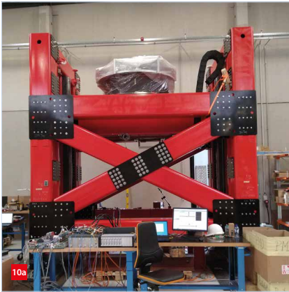
Support structure and rotary table with axial and radial air bearings for an X-ray imaging machine. (a) Overview. (b) Close-up.
