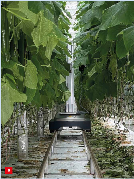
Prototype leaf-cutting robot by VDL CropTeq.
