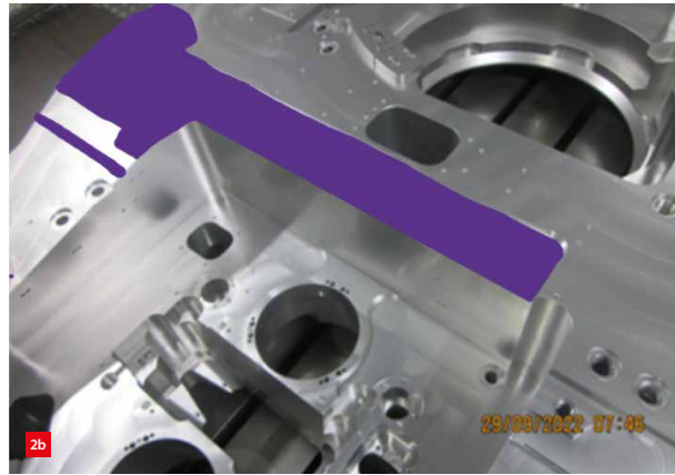
Analysis of the changes required to make the DUV metrology frame applicable for re-use. The orange colour indicates potential interface plates as lessons learned for future designs. Additional features needed are marked by the purple colour.
