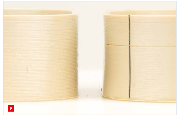
The printed part on the left demonstrates that shrink compensation prevents deformations such as curved surfaces (right).
