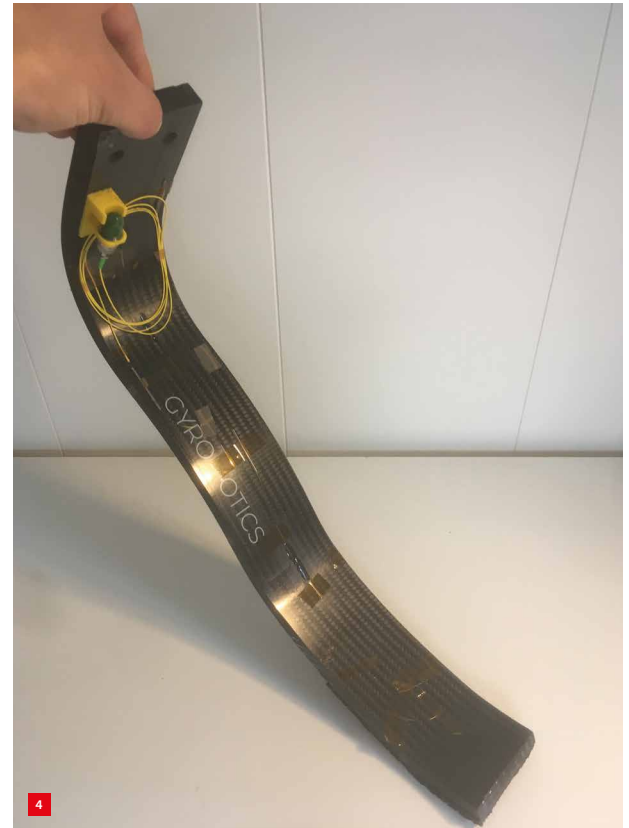
ArcX Extreme prototype instrumented with FBG sensors.
