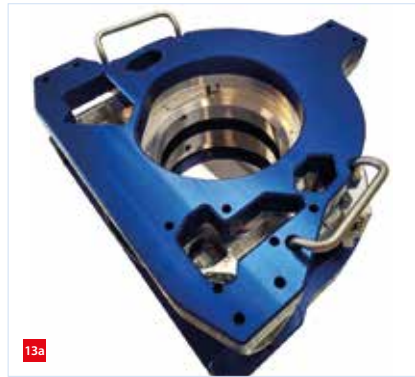
Assembled sensor. The sensor ring (aluminium colour) is suspended from the top frame (blue), which stands on the bottom frame (blue), which in turn carries a 300-mm wafer (only the edge visible on the left). (a) Rendering. (b) Realisation.
