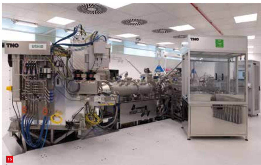
Overview of the EUV Beam Line 2 (EBL2).
