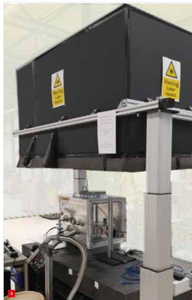
Experimental set-up to study the particle-gas interaction with the possibility to control pressure, temperature and temperature gradient. The photo shows all the main components of the set-up: the vacuum chamber (in the middle) on top of an optical table, and a special cover (black box above the chamber) closing the chamber during the experiment for safety and optical background reduction [5].
