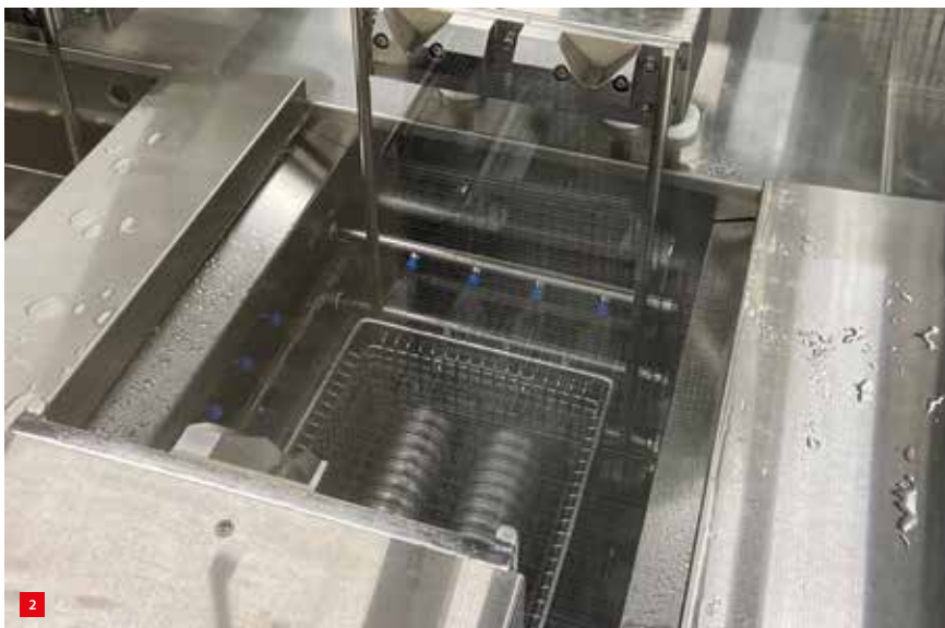
2 An immersion-type spray rinse tank sprays off the parts as they exit the bath for an improved rinsing result. (Photo: Philips Medical Systems)
