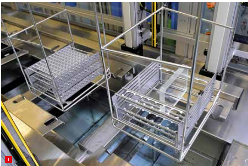
Round and flat optical components are increasingly made from acid-sensitive glass. To avoid glass corrosion with these sensitive materials, appropriately designed cleaning and water treatment systems and processes - including software - are indispensable. (Photo: Zeiss)
