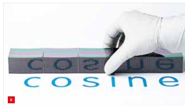
Five stacks of SPO mirror plates produced for a test pilot production run. Each stack consists of 35 mirror plates. The colour sheen on top of the stacks is caused by the wedge shape of the plates, which aligns all plates to reflect X-rays to a common focal point. (Photo: cosine)
