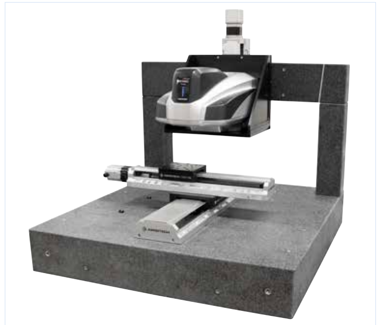
Integration of the Keyence wide-area 3D measurement system VR5000 into an Aerotech positioning system.
