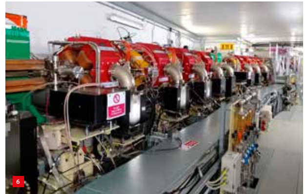
Accelerating and beam aligning magnets for synchrotron storage ring.
