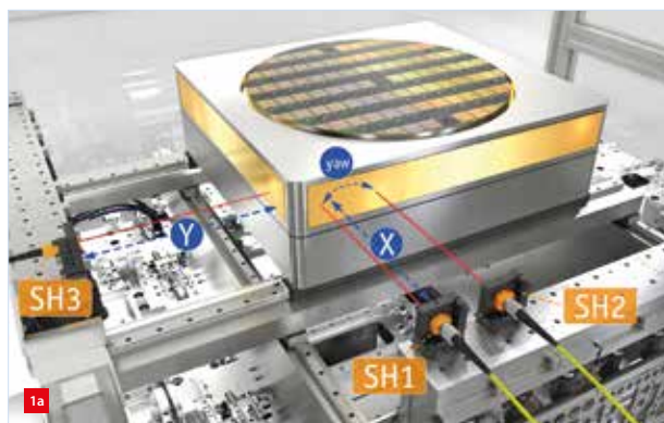
Two xy-stage control application examples using the IDS3010 sensor. (a) Two sensor heads (SH1 and SH2) measure the displacement on the yz-mirror surface. The SinCos signal of SH1 is used for closed-loop control of the x-axis. SH1 and SH2 are horizontally separated by 40 mm, therefore the yaw rotation can be calculated and utilised as the real-time compensation for a 4-DoF set-up. The third sensor head (SH3) controls the y-axis.
