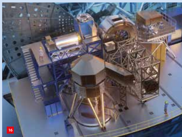
Render of the ELT and the Nasmyth platform, showing, from left to right, the instruments HARMONI, MICADO, MAORY and METIS. The platform is the same size as a basketball court. (Image credit: ESO)
