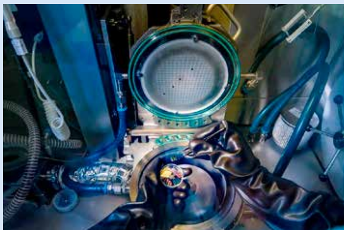
A look inside the machine in which nanowires were grown that made it possible for silicon to emit light. This TU/e finding was named 'Breakthrough of the Year' by PhysicsWorld last year. (Photo: Nando Harmsen)
