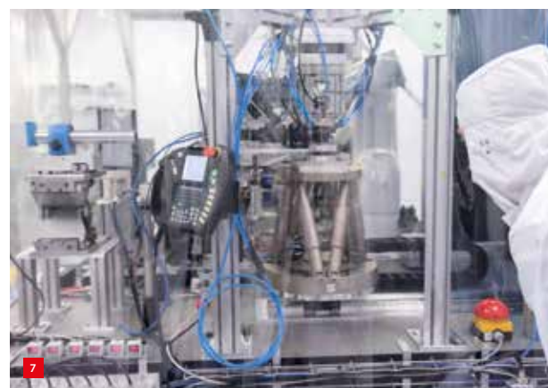
Custom robots for the assembly of SPO mirror stacks in the cleanrooms at cosine. Inside the down-flow tent, the mandrel is mounted on a hexapod, on which the stack is assembled by the robot. Four stacking robots are operational for development in preparation for mass production. (Photo: cosine)
