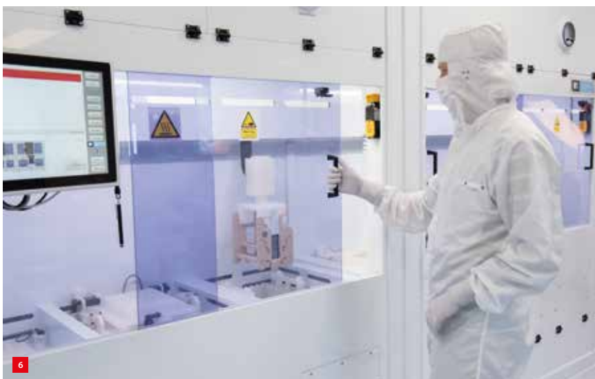
The highly automated wetbench at cosine, where SPO plates are cleaned and activated prior to being assembled in mirror stacks. This prevents contamination that would reduce the bond strength of the plates, while particles trapped between bonded plates would significantly degrade the optical quality. (Photo: cosine)
