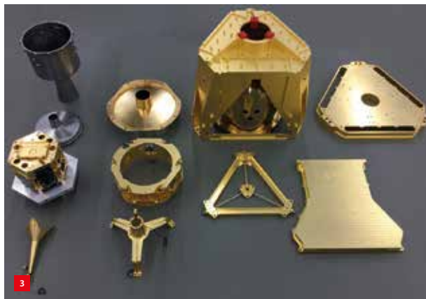
Parts of the FPA Demonstration Model. Upper left is the niobium shield, middle left the 50-mK assembly, and lower left the cold finger; the second row from the left shows the three parts of the 300-mK stage; on the right half, the 2-K parts, with the triangular Kevlar suspension (one of three).
