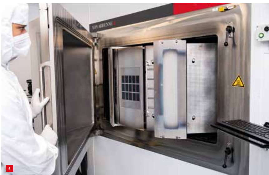
Loading of SPO plates in the magnetron sputtering system for coating with iridium. Due to its high atomic number, the iridium layer increases the fraction of X-ray photons that are reflected by the mirror. This is especially important at photon energies in excess of 2 keV. The coating, therefore, extends the energy range of the telescope. (Photo: cosine)
