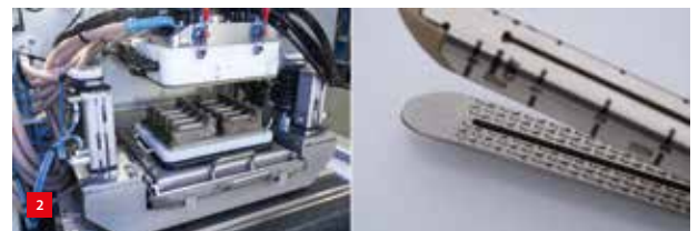
PECM is used, among other things, for manufacturing medical devices, in this case a stapler for closing wounds with staples. Workpieces are microstructured in a multiple tool with an imaging accuracy of < 20 µm and a surface quality of R_a < 0.1 \mu\text{m} . (Image: EMAG ECM)
