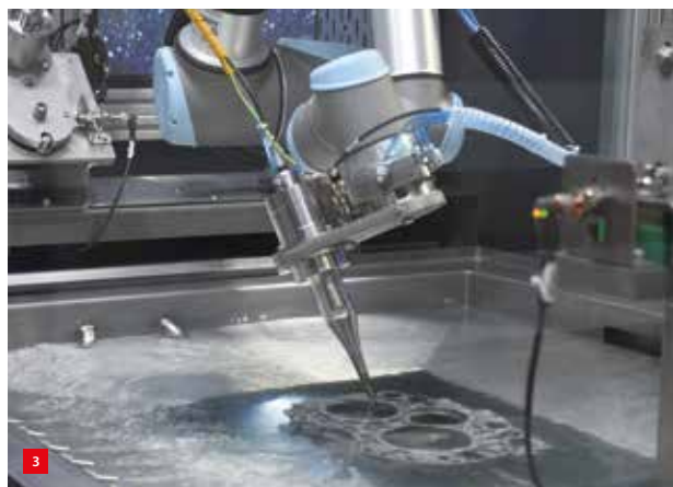
Ultrasonic deburring can also be used to reliably remove internal and hidden burrs. Parts are cleaned and deburred at the same time. (Image: Doris Schulz)
