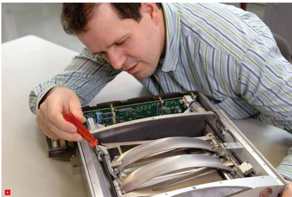
Senior designer Michel Loos showing the construction of the collimator with two curved shutter blades.
