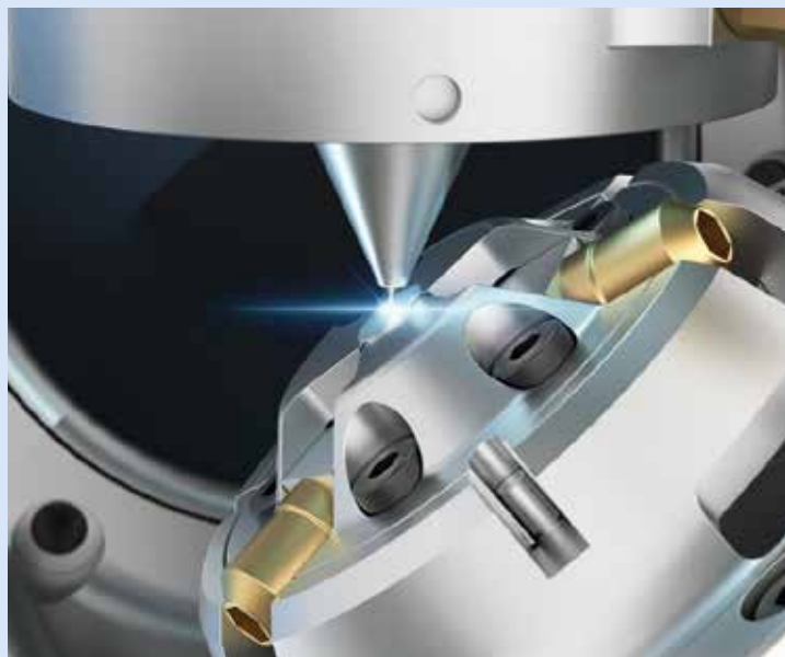
Precision microdrilling of an injection nozzle (with femtosecond laser and 5-axis scan system). (Image: stoba)
