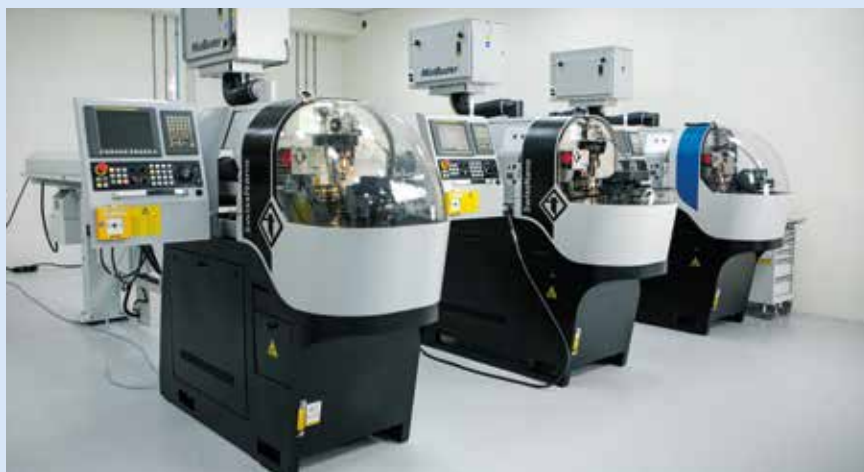
Exakt has Swiss-type CNC precision lathes in-house for turning extremely small parts with highest accuracy.
