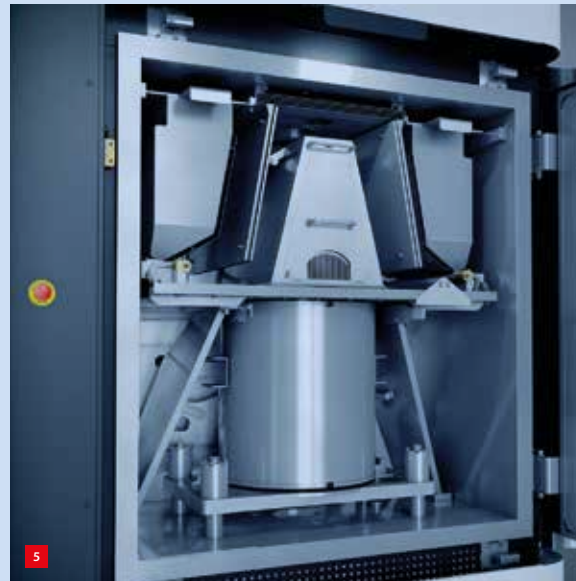
The vacuum chamber inside an Arcam printing machine.
