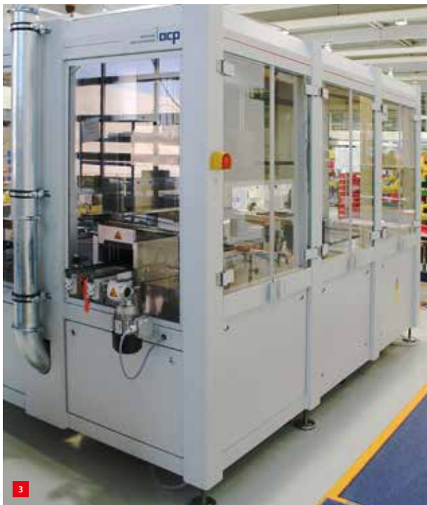
The modular concept allows different processing steps to be integrated into the system, such as separation, alignment, and cleaning, as well as electronic function tests.
