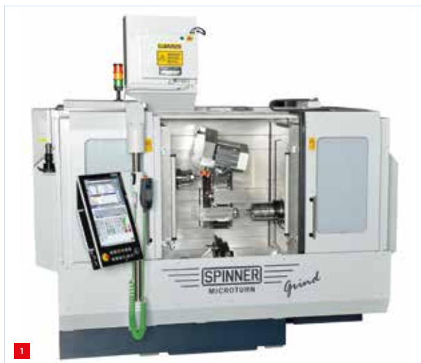
The Spinner Microturn Grind machining centre with open safety door.
