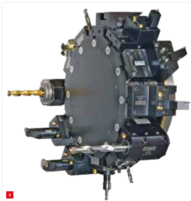
The indexing turret for holding twelve tools, motor driven when necessary, with BMT45 coupling interfaces.
