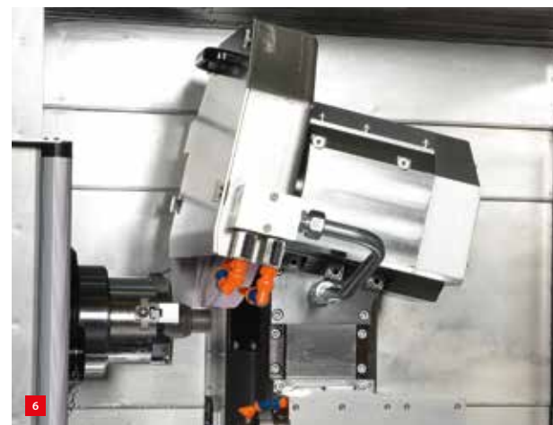
The external grinding wheel with a maximum outside diameter of 400 mm.
