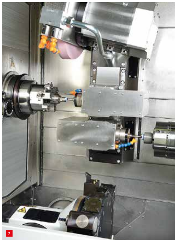
The pair of spindles for internal grinding with either left or right orientation.
