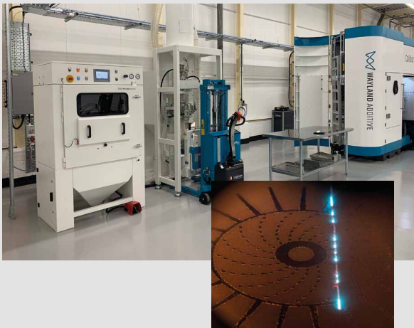
A complete Wayland Additive set-up, with the Calibur3 eBeam PBF system on the right. The inset shows the machine in action.
