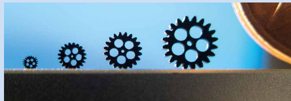
The Nano Dimension Fabrica 2.0 and some typical printed products; on the right, a 2 eurocent coin for comparison.
