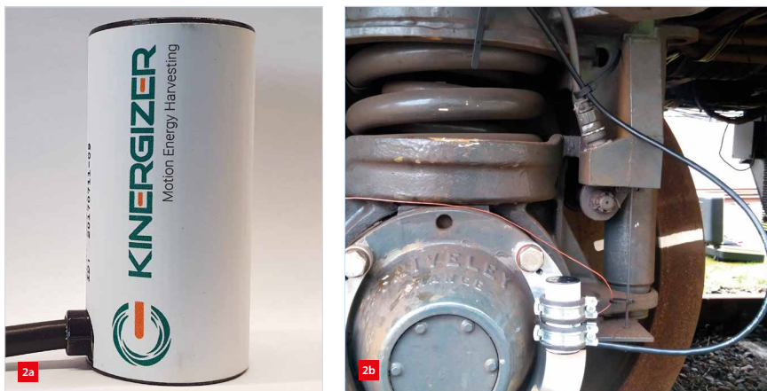
Application example of Kinergizer's energy-harvesting solution. (a) The Hiper-D energy harvester (ø35 mm, 75 mm height, 90 g mass, 1-5 mW power). (b) Mounted to a train bogie axle box.
