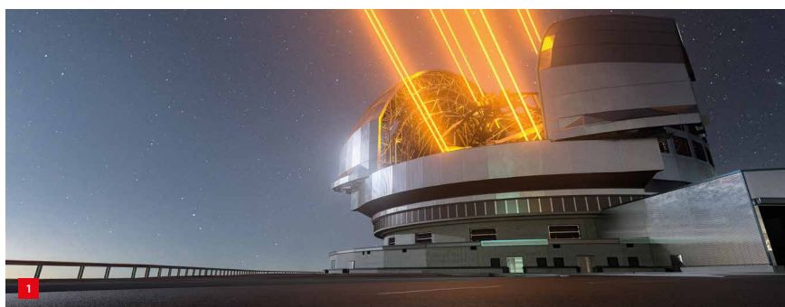
Artist's impression of ESO's Extremely Large Telescope (ELT), which will be the world's biggest 'eye on the sky' when it achieves 'first light' later this decade. Eight LPS systems will create artificial guide stars for measuring how distorted light is due to turbulence in the Earth's atmosphere. ELT's deformable M4 mirror will adjust its shape in real time to compensate for these changes in the atmosphere, helping to produce images that are 16 times sharper than those of the Hubble Space Telescope. (Image credit: ESO)
