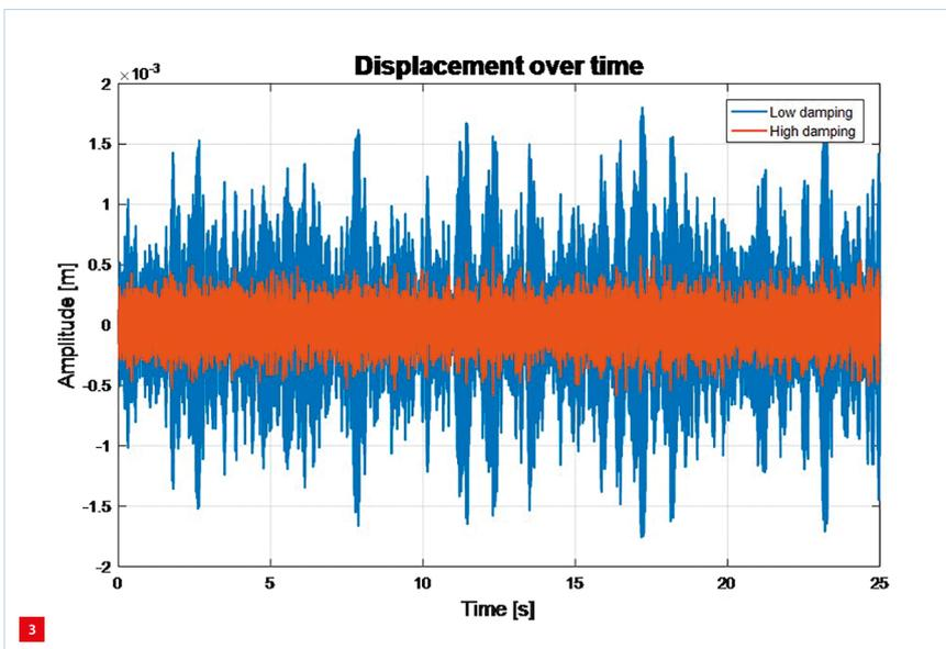
Time domain simulations that clearly show the difference in displacement between the system with low damping (blue) and high damping (red).
