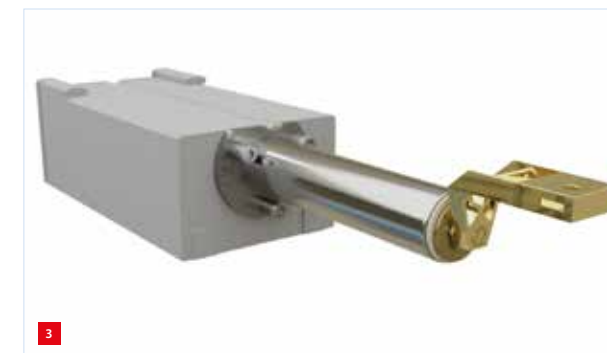
Design of the cryogenic micro-cooler. On the right, a still from an animation of the cooler mounted on a moving 5-DoF manipulation stage.
