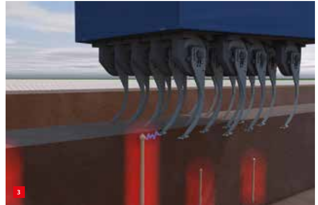
Detection trigger at close proximity of an asparagus spear to a probe.
