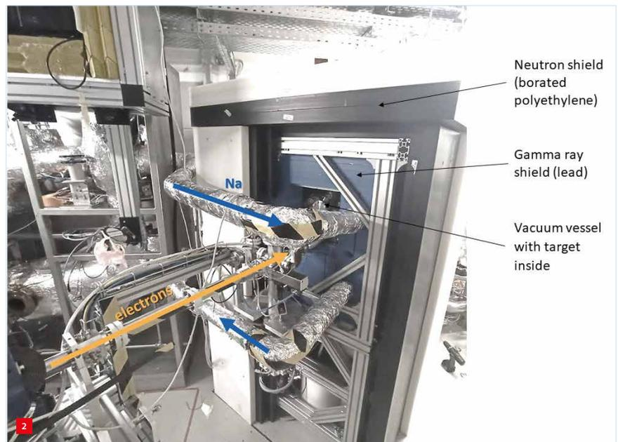
The 1:1,000 miniature version of the SMART exposure cell. It was installed at the ELBE electron accelerator at HZDR Dresden-Rossendorf (one of Germany's Big Science facilities). Power density, Na cooling and target materials are representative of the SMART target.
