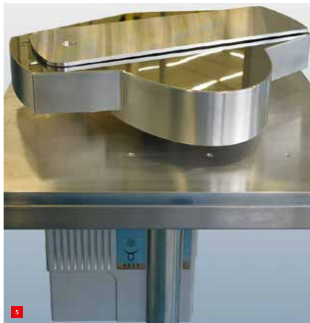
Example of a wafer-handling robot containing a linear guide (Asys Micro).
