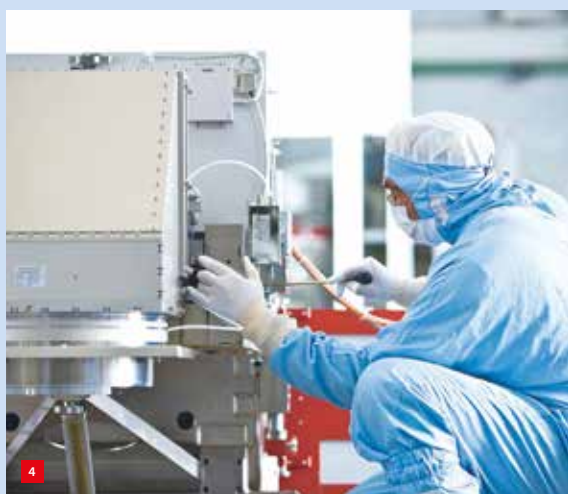
An ASML technician working on a wafer scanner in a high-grade cleanroom. (Photo courtesy of ASML)
