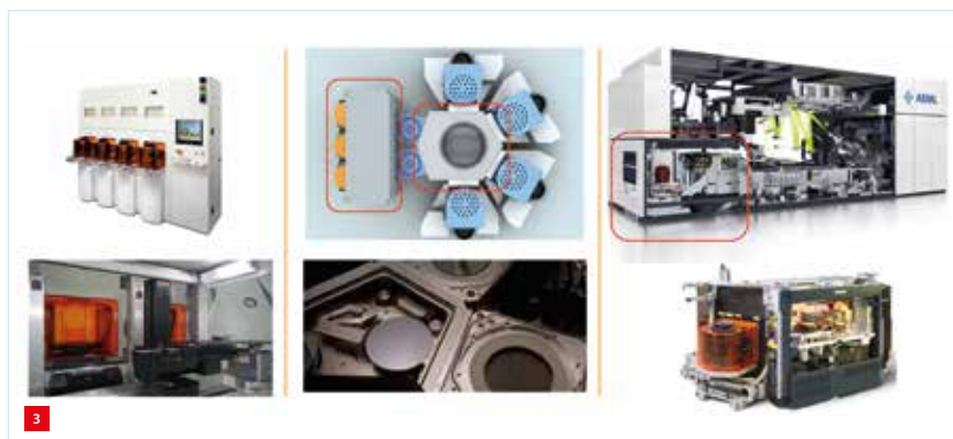
Three common wafer-handling system architectures, from left to right: Kensington Laboratories (top) and Brooks Automation (bottom); Applied Materials; ASML. See text for further explanation.
