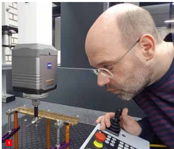
Nobby Assmann with his Zeiss Contura coordinate measuring machine with VAST XT Gold active scanning head.
