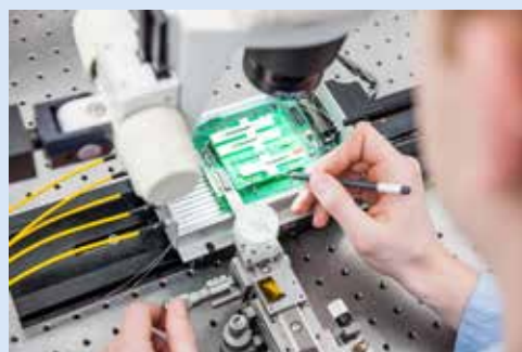
Production of a fibre switch with multimode fibres.
