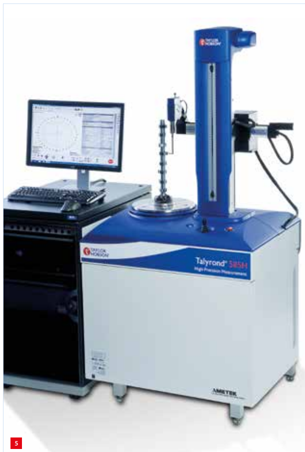
A Talyrond roundness tester with an extreme radial air-bearing accuracy. (Photo courtesy of Taylor Hobson).
