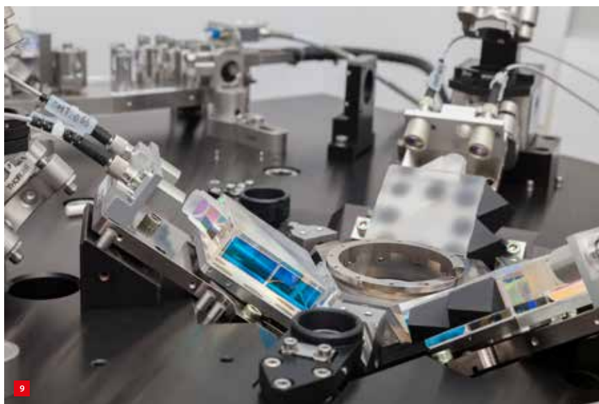
Close-up of the LDR-AFM's positioning stage. Right of centre is the hexapod positioning stage with a hole for accommodating the AFM head. Also visible are the laser interferometers consisting of fibres with collimation optics (top-left, top-right), beam-splitters (large glass blocks with blue-coloured rectangles due to a reflective dielectric coating on two of the mirrors), and mirrors attached to the positioning stage. (Photo: Henri Werij)
