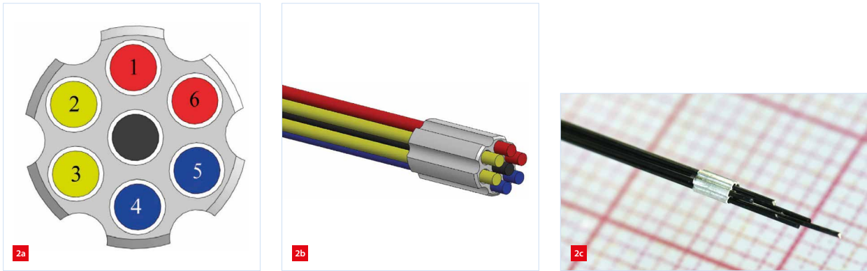
First design of an ovipositor-inspired needle. (a) Cross-section of the flower-shaped ring, with a central hole to which the central wire is glued and six peripheral holes through which the six other wires can slide back and forth. (b) Initial position of the wires. (c) Prototype, showing the tip of the needle with the ring, and some of the wires moved forward.
