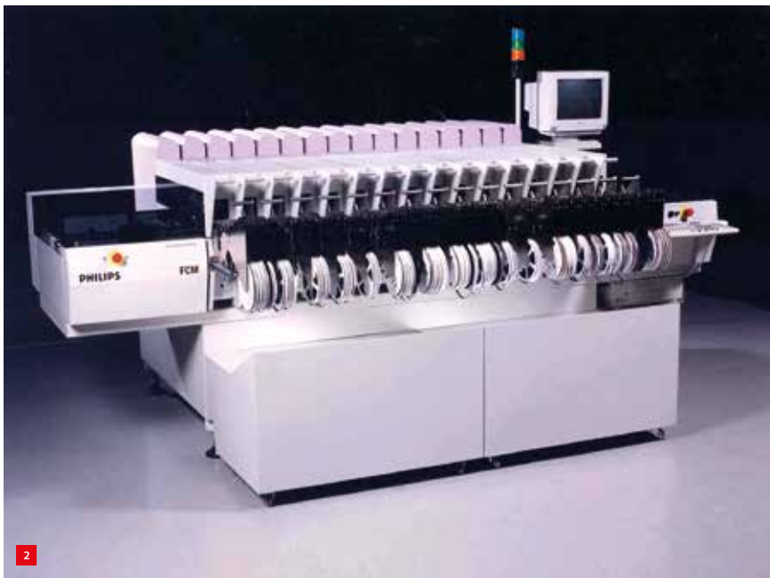
In the 1980s, Philips CFT started developing machines for mounting smd's (surface mounted devices) on pcb's. The revolutionary FCM-II (Fast Component Mounter) by Philips EMT featured 16 placement robots working in parallel. Hans van de Rijdt's contribution was the design of the pcb transport module, among other things. More than 1,000 of these machines were produced.
