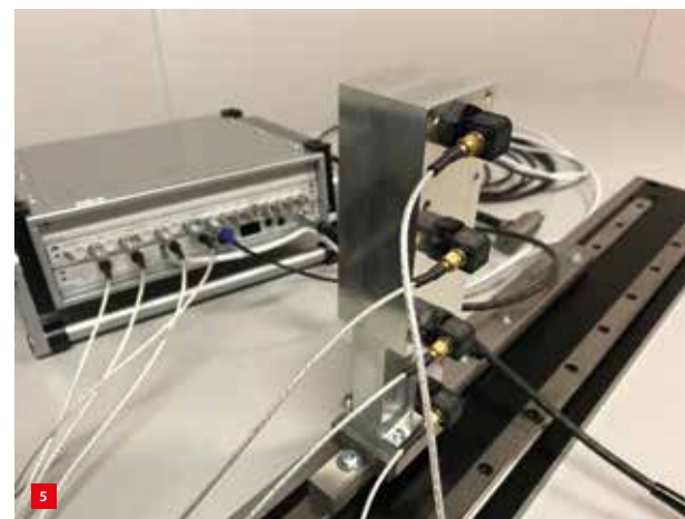
Hammer impact testing was applied to the bearings to identify their stiffness in the relevant degrees of freedom.
