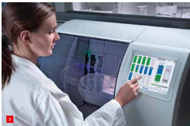
The Philips Ultra-Fast Digital Pathology Scanner, combining exceptional image quality with high speed and throughput. All sample slides are scanned at high resolution, providing visibility to cellular detail, using multi-sensor technology and parallel processing.
