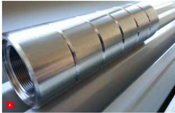
A cylindrical workpiece with recessions machined with free-jet ECM technology.
