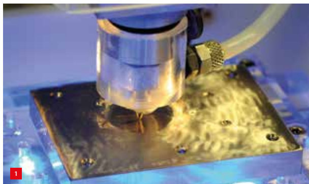
The TU Chemnitz free-jet ECM set-up with a fixed electrode and a movable workpiece on a high-precision XYZ-stage.
