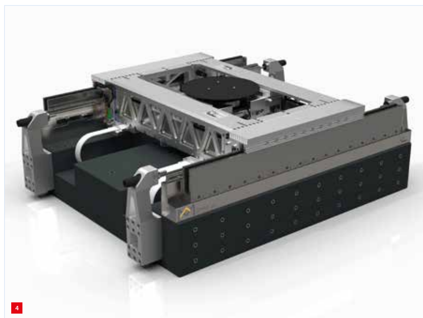
The resulting design: a stage featuring a rigid granite base plate, linear motors and linear bearings for each axis, and a Zθ-module in the centre of the XY-axes. Wafers can be placed on the black circular plate on top of the Zθ-module.
