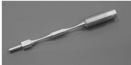
Figure 4.5: Reinforced strut for prism block alignment
