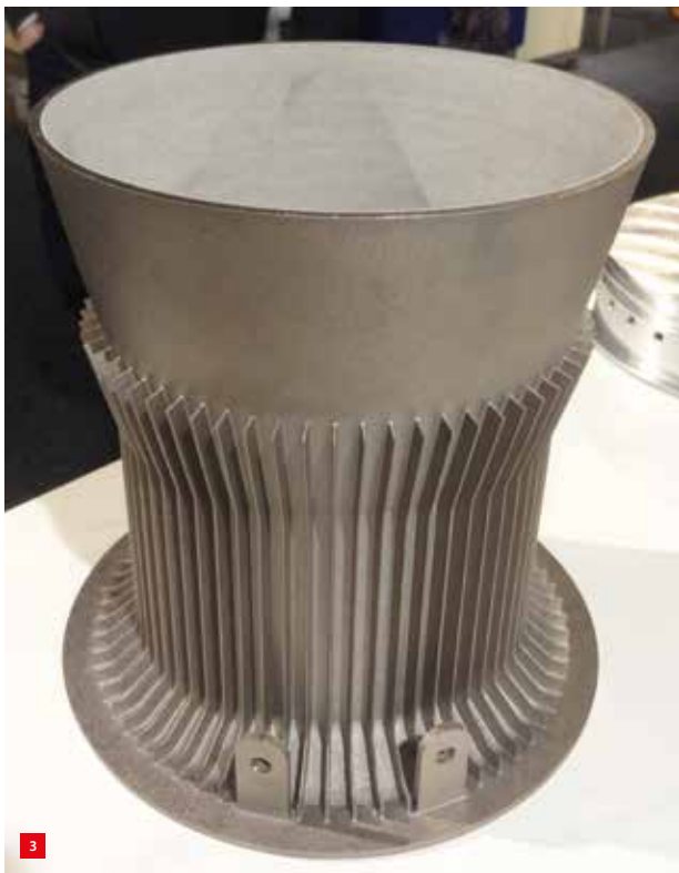
A 3D-printed rocket nozzle made from titanium, designed by the DARE team from Delft University of Technology.
