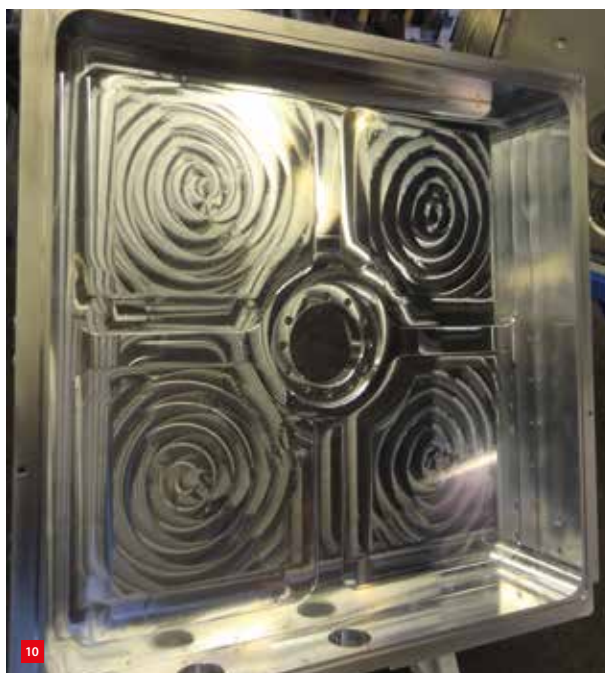
A part of a vacuum chamber produced by Vernooij Vacuum Engineering, machined from a massive block of aluminium.
