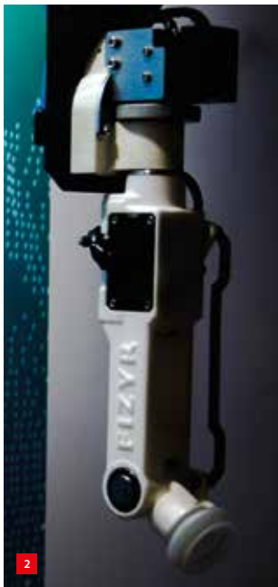
An example of a flexible gripper, designed by Fizyr for 3D-printing.
