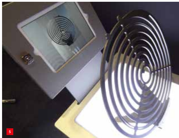
A stainless steel workpiece made by Lucassen Watersnijtechniek using water cutting technology.
