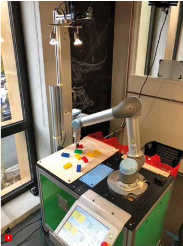
Set-up with camera in the top and illumination of the Duplo blocks.
