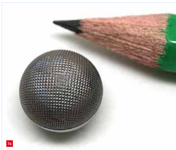
Microscale laser ablation by Lightmotif. (a) A texture with tiny pits made with an ultrashort pulse-laser. (b) The Lightmotif 5-axis laser micromachining system.
