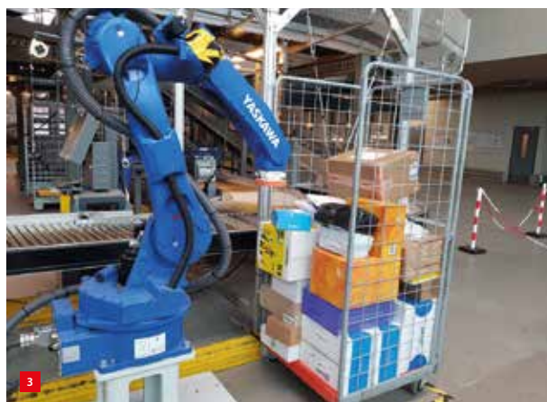
A typical application environment for Fizyr's AI-supported vision-based picking software: picking parcels from a roller container, to place them on a conveyor (or vice versa).
