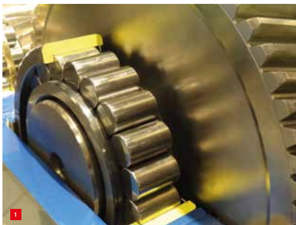
A cageless Schaeffler high-load roller bearing in a gearbox for windmills.
