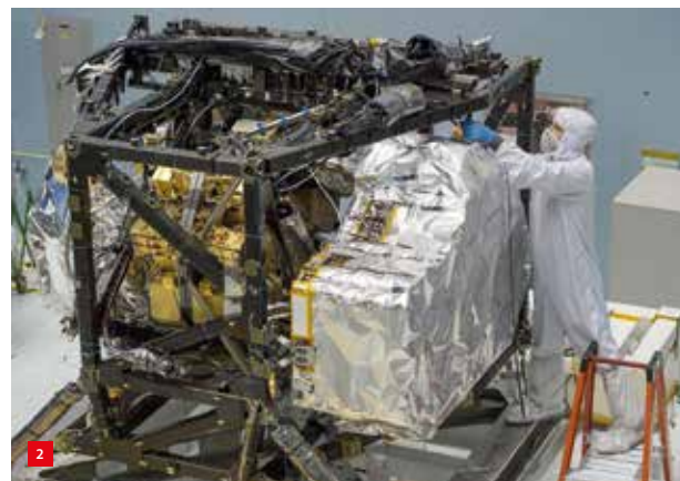
JWST's Integrated Instrument Science Module with its instruments: MIRI (left, wrapped in aluminium-coated multi-layer insulation), in the centre NIRCam at the front and FGS in the back, and NIRSpec (right). (Image: NASA)
