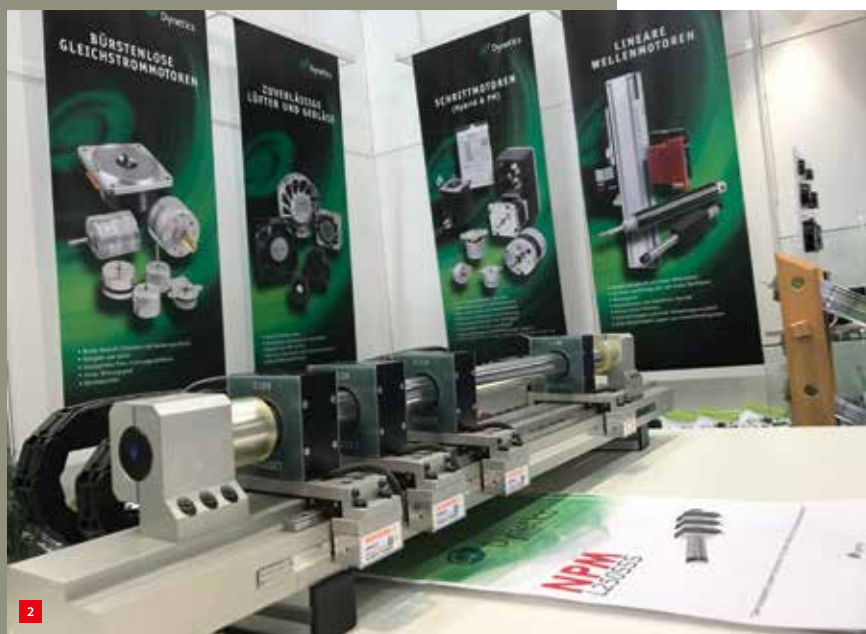
Compact linear servo motors supplied by Dynetics for high-power-density applications.
