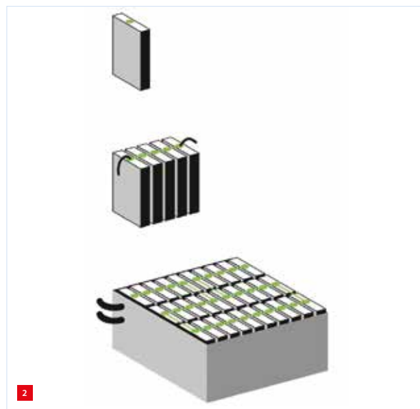
Packing individual battery cells into modules, which are combined in battery packs to be mounted into vehicles.
