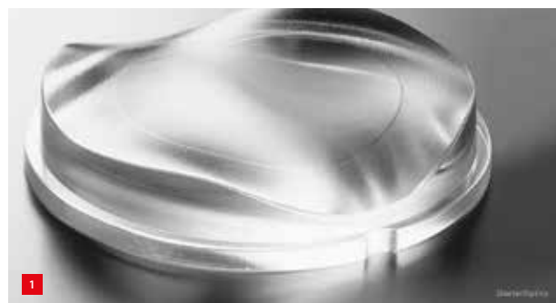
It's not only possible to measure aspheres, but also so-called freeforms. (Source: Docter Optics SE)
