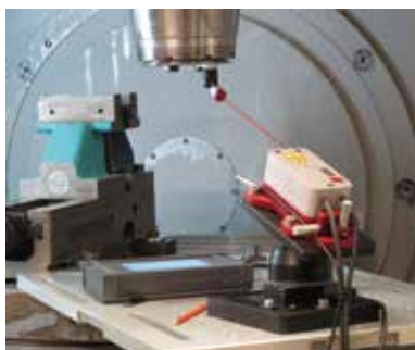
The compact SP-NG interferometer for a diagonal measurement in a machining centre.
