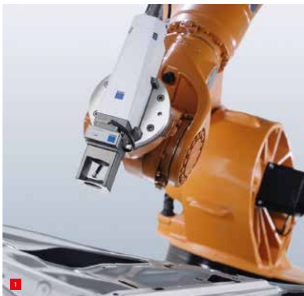
Welding a steel sheet part with a Trumpf laser.
