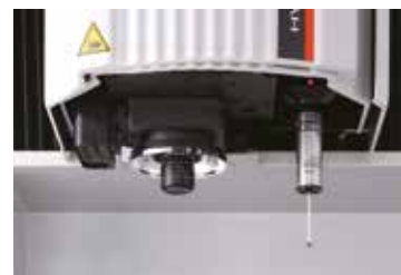
The MiSCAN multi-sensor vision system.
