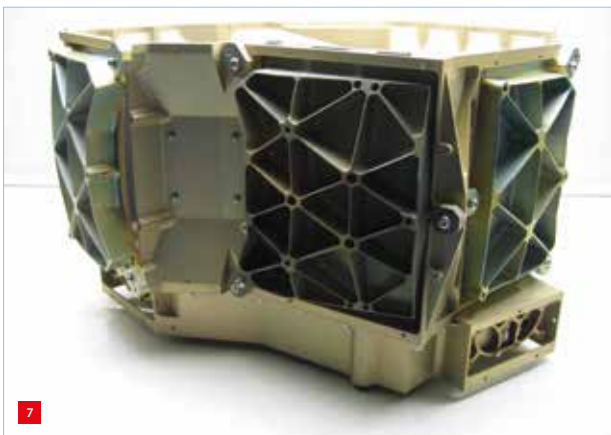
The SW arm. The open-back light-weighted mirrors are mounted with three bolts and two pins each. The largest optics are assembled onto the central support (from left to right: M1-2, M3 and M1-1) and the two (identical) collimator mirrors in the bottom (left and right). (Image: NOVA-ASTRON)
