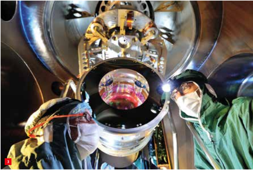
Input mirror of Advanced Virgo, suspended from a super-attenuator. The mirror is the last element of a chain of horizontal and vertical vibration isolators, all housed in a 10-m-high ultra-high vacuum tower. The black ring in front of the mirror is a light baffle, meant to prevent stray light to re-enter the interferometer. On the photo Maurizio Perciballi (left) and Ettore Majorana. (Photo: Maurizio Perciballi)
