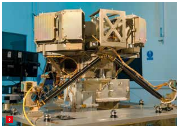
MIRI with the spectrometer (top), the deck that connects the modules with the CRFP struts (middle), and the imager and pick-off mirror assembly (bottom). (Image: MIRI consortium/STFC/RAL Space)
