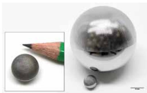
A 10-mm diameter steel sphere with a pyramid texture ( 0.2 \times 0.2 mm raster, 100 \mu m high). Behind that a 50 mm diameter steel sphere with a negative pyramid texture ( 0.5 \times 0.5 mm raster, 40 \mu m deep).
