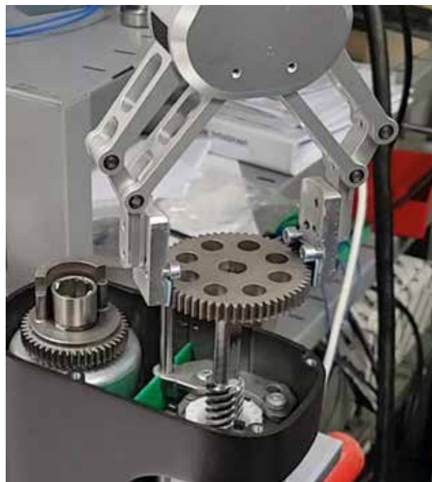
3 Søren Peter Johansen of DTI advises avoiding full automation. Here, components previously placed on the table by an operator are picked up by a vision-driven collaborative robot for assembly. (Photos: DTI)
