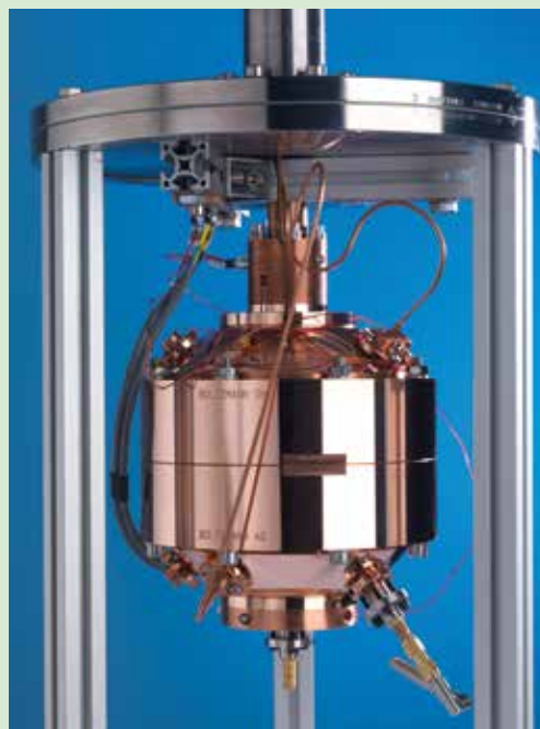
■ Resonator used for acoustic thermometry. (Courtesy: NPL)
