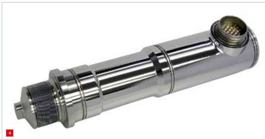
4 A stepping actuator with a resolution of 2.5 nm designed by JPE for UHV applications. The hermetically closed inside houses proven technology with a screw spindle and stepper motor.
