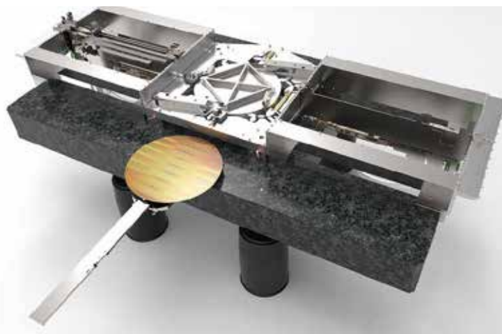
■ Nearfield Instruments' solution for making IC inspection up to 1,000 times faster is AFM parallelisation, achieved by miniaturising the AFM and operating many of them simultaneously.
