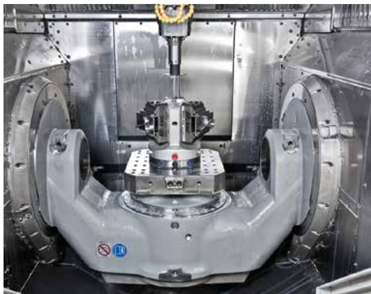
■ The working area of a C 22 U high-performance five-axis machining centre featuring the 320 mm diameter NC swivelling rotary table with a multi-clamp system installed on it. (Copyright Hermle)
