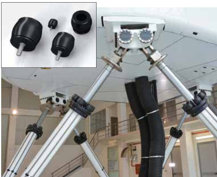
■ ACE's TUBUS TA dampers (see inset) attached to an E2M motion system.
