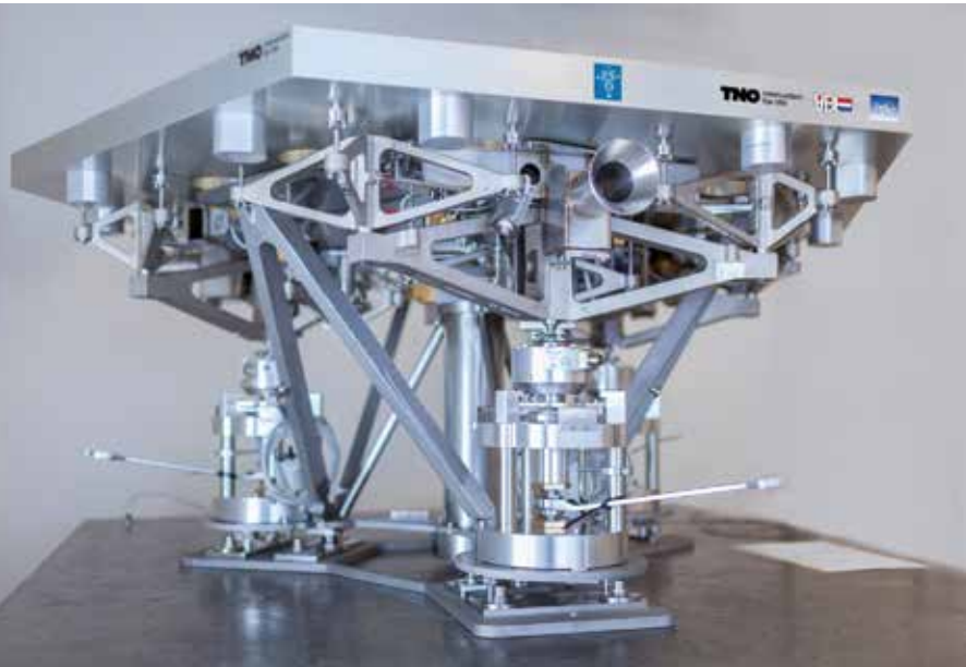
Support structure for a single mirror of the European Extremely Large Telescope (E-ELT) which contains 798 mirrors in total. Developed in close cooperation between VDL ETG, TNO and TU/e.
