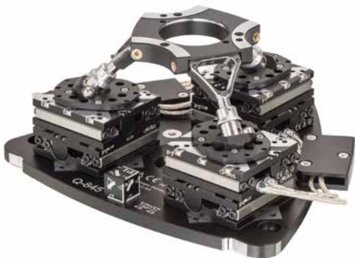
■ High precision and high stiffness: the SpaceFab Q-845 parallel-kinematic positioning system can position loads of up to 1 kg in 6 DoFs with nanometer precision and hold them in a stable position.
