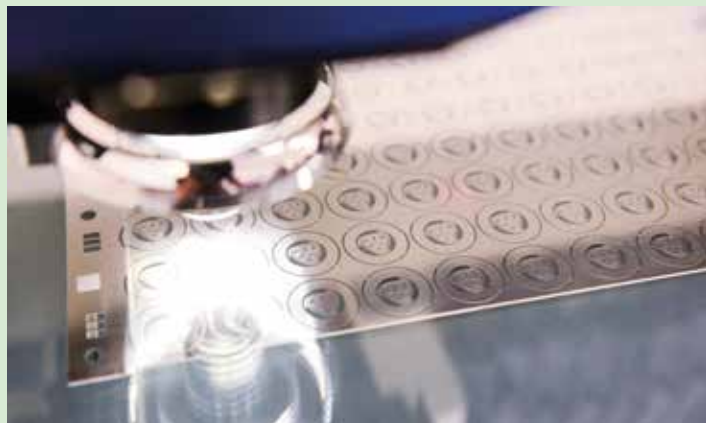
■ Precision Micro supplies photo-etched flexures used in gasoline direct injection systems.
