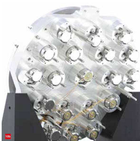
10 The demonstrator. (a) Front view (b) Back view with (dummy) actuator modules.
