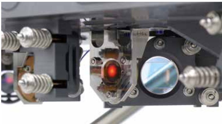
■ Detail of the Gaia BAM space interferometer; also read the article on page 28 ff. (Photo: TNO/Fred Kamphues)
