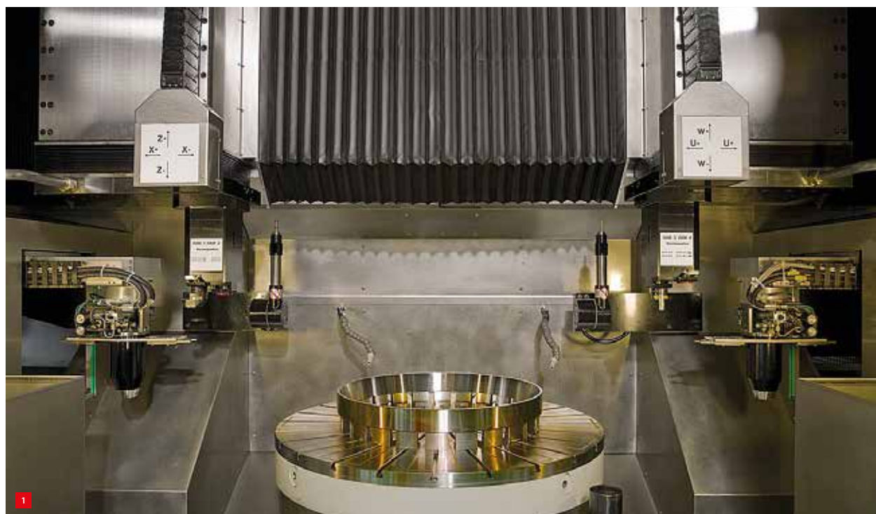
1 The turntable of the Hembrug vertical hydrostatic turning machine Mikroturm V4 with a run-out accuracy of 0.2 µm. This machine can be equipped with a grinding or a polishing unit.
