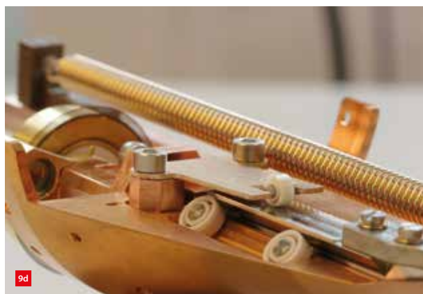
9 Realised MFSR. (a) Without caps. (b) With caps. (c) The secondary (left) and the primary wheel. (d) The rack running through ceramic ( ZrO_2 ) bearings in a V-shape configuration, with the rack preload spring on top; in the background the tension spring which preloads the primary wheel. (e) The PiezoKnob actuator with fibre-optic encoder.
