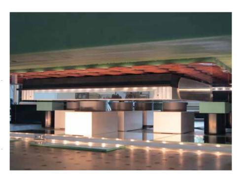
■ The Ceiling Robot is the world's first 'flying' planar motor in which a robotic platform is magnetically and contactlessly suspended underneath a ceiling. A prototype of this unique and complex mechatronic system was constructed in the TU/e research group of prof. E.A. Lomonova.
