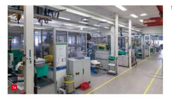
Production facilities at Philips Ceramics Uden. (a) Mechanised production lines for ceramic injection moulding. (b) Industrial furnaces operated under hydrogen condition ensure controlled sintering conditions.
