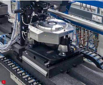
combined with high-resolution optical linear encoders. When driven accordingly, this allows closed-loop step sizes of a few nanometers. The precision crossed-roller guides and ball screws used also contribute to the high positioning accuracy.
