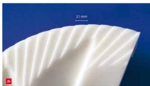
standard compounds can be realised by adjusting feedstock composition, e.g. binder optimisation to enable the injection moulding of thin-walled products (Figure 4) or adding dopes to the feedstock compound to improve mechanical product characteristics.
