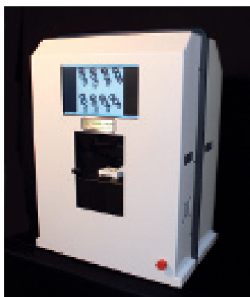
■ The CGI Pearl 900 machine and an image from the CGI colour mapping software used to compare a 3-way connector scanned part data with the original CAD design. Green areas are within tolerance, red and blue are too big and too small respectively.
