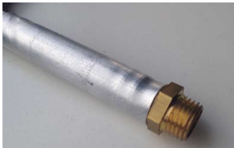
Figure 5. An example of a connection made with electromagnetic forming.
