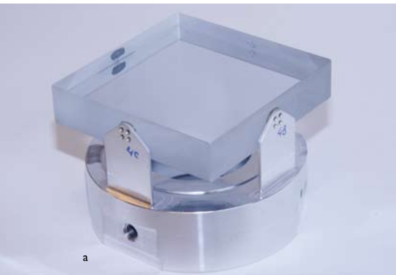
Figure 4. Breadboards of the TROPOMI mount baseline showing aluminium leaf springs bonded to a fused silica component. The thick baseplates contain a diamond turned reference for interferometric stability measurements. The dark bond spots are clearly visible. Please note that the optical components are different in size and that the magnification of both photos is different.
