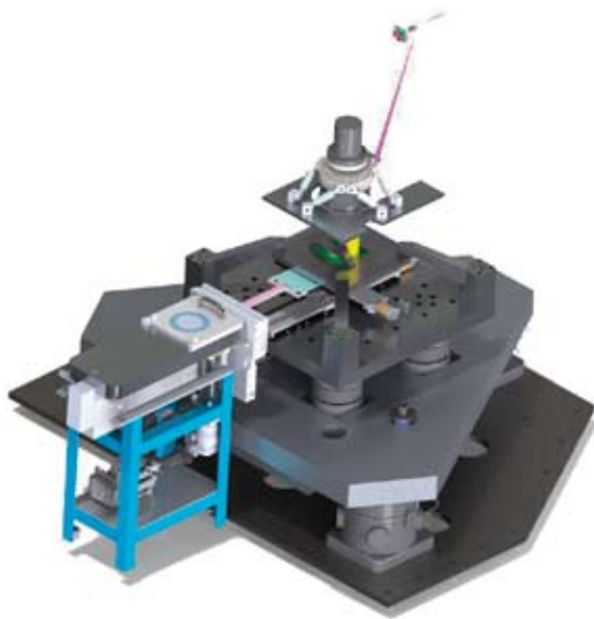
Figure 2. The synchrotron-based SHARP EUV mask microscope isolates the critical mask and zoneplate-lens stages inside a vacuum test chamber.
