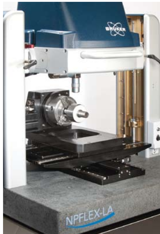
Figure 3. Measurement of shaft lead angle with a 3D optical microscope.
