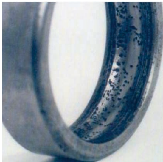
Figure 5. Example of bearing corrosion as a result of transient arcing.
