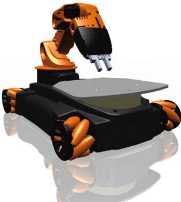
Figure 2. One the robots featured at the RoboNED plaza was the KUKA youBot. This robot was developed by German industrial robotics manufacturer KUKA Robotics as a mobile manipulator for education and research.
