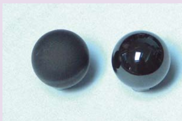
Figure 8. 12.7-mm diamond-coated & polished full sphere; \text{Si}_3\text{N}_4 material (in development).
