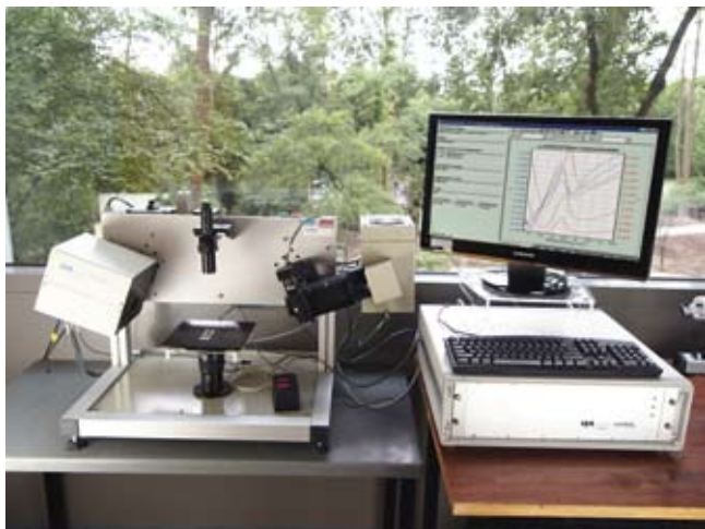
Figure 2. The ellipsometer in the MATinspired lab can accurately determine the thickness of thin coatings.
