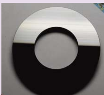
Figure 7. 100-mm diameter diamond-coated & polished ring ( < 1 fringe); underlying material of SiC.
